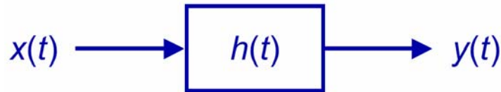
Figure 3. Model of a linear system [20].
