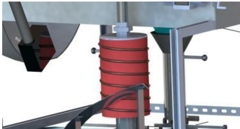
Figure 13: Urine Disinfection Coil on Reactor Hood (Weimer, 2013)
