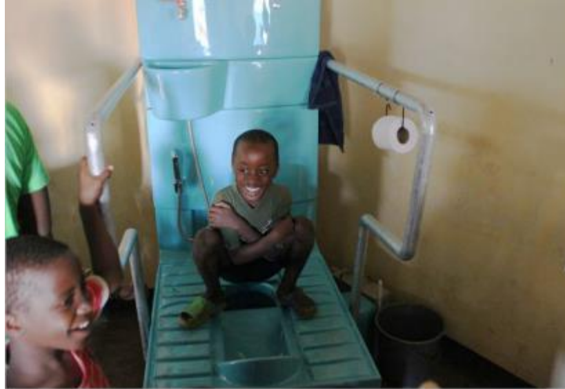
Figure 19: Child testing the Blue Diversion Toilet during field test in Kampala, Uganda (Eawag, 2015)
