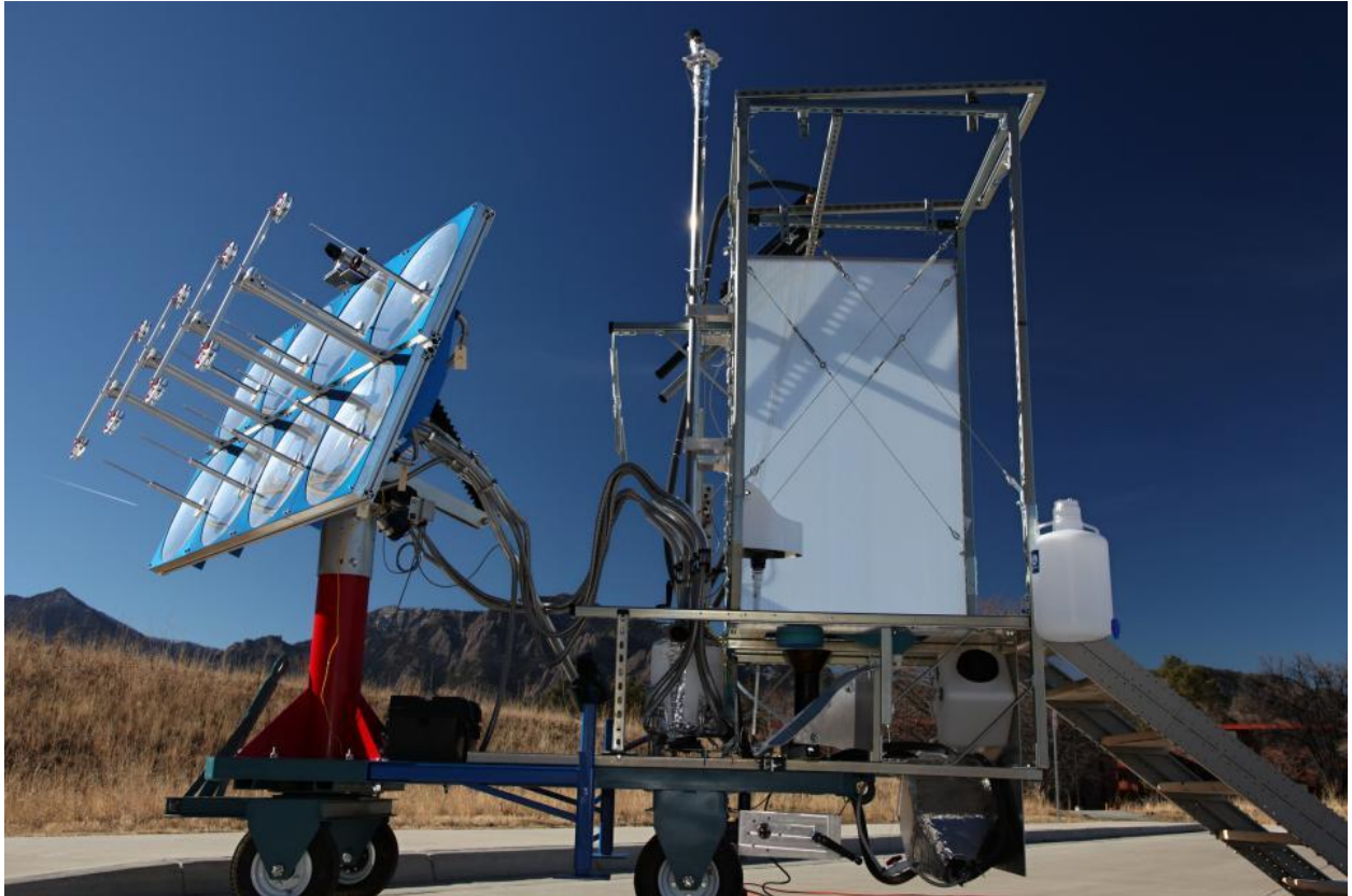
Figure 25: Sol-Char Toilet Phase I Design (University of Colorado Boulder, 2015)
