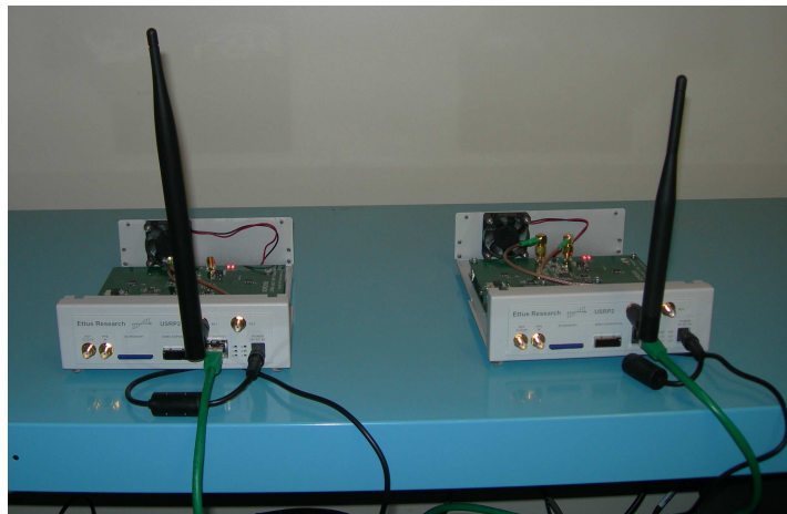
Figure 4.13: Two USRP 2.0 radios set up to transmit and receive in the WPI Wireless Innovation Lab.
