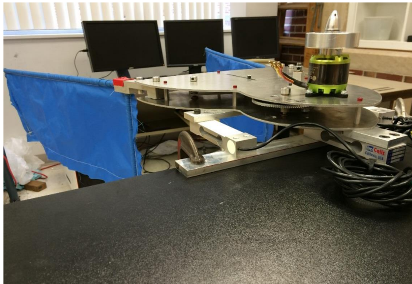
Figure 13: Side view of ornithopter prototype hard mounted to the sensor platform
