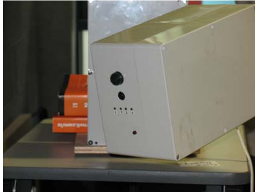
Figure 27: Camera node with the enclosure.
