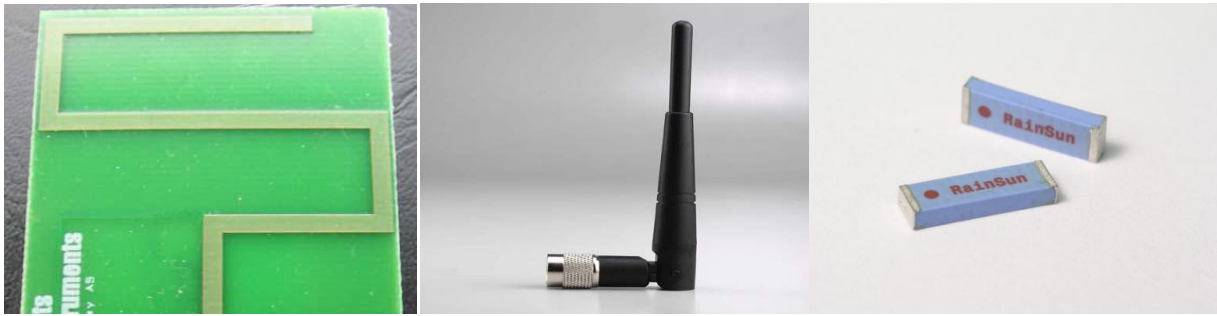
Figure 22 PCB (left), Whip (middle), and Chip antennas (right) (Texas Instruments, 2009)
