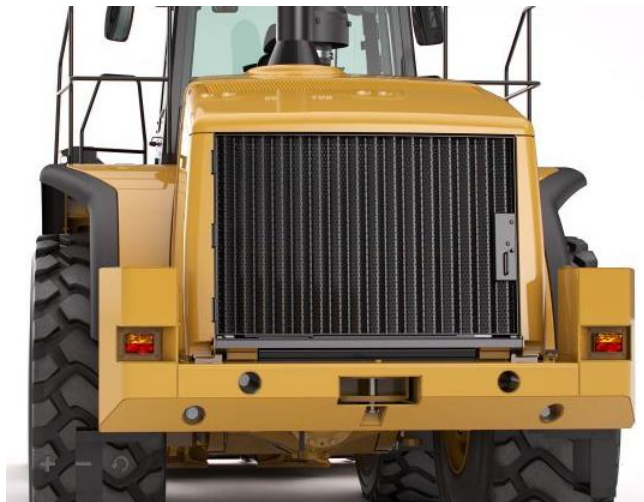
Figure 4: 980H counterweight and rear signal lights
