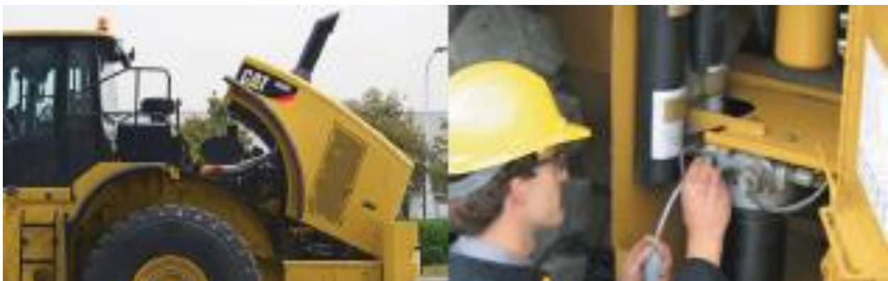
Figure 2: Tilted engine hood and side access doors
