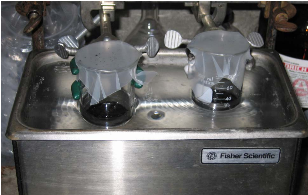
Picture 3.1 Sonication of catalyst ink
