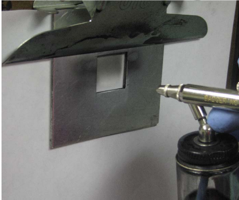
Picture 3.5 Applying catalyst slurry directly to the membrane with airbrush.
