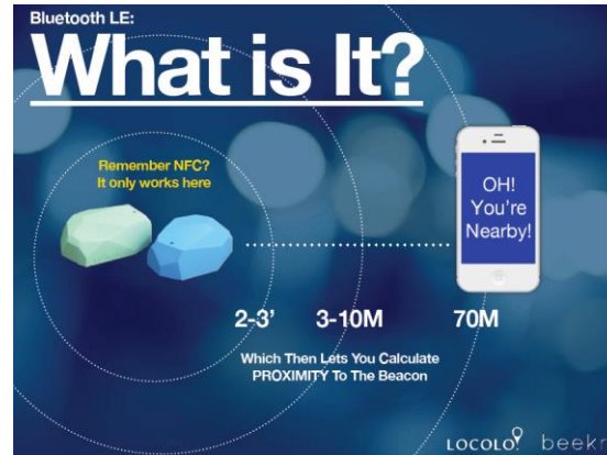
Figure 2.3: Example of How iBeacon and Smart Devices Interact
