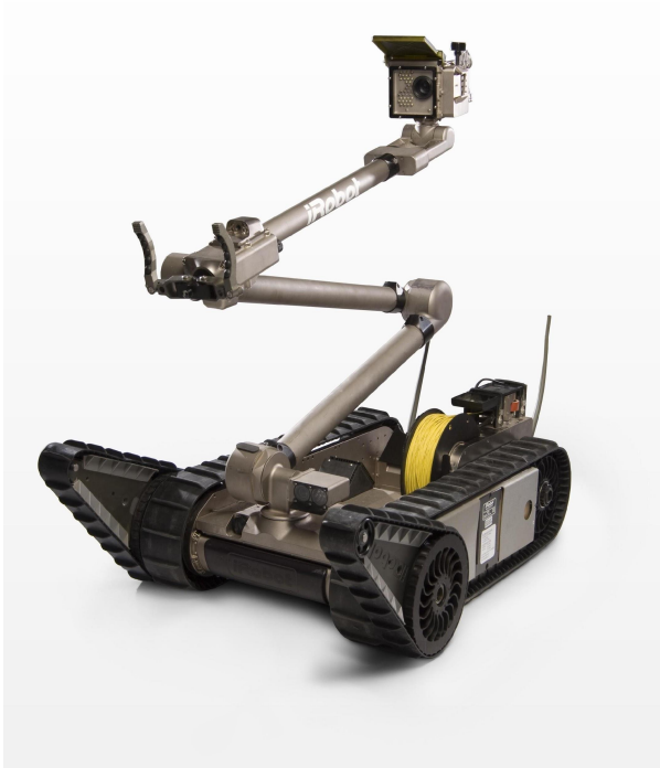
Figure 1 - iRobot PackBot with Explosive Ordnance Disposal (EOD) Arm
