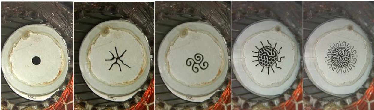
Figure 1.1: This figure, taken from http://www.eecs.mit.edu/grad/area4/subjects.html , demonstrates some major features seen in thin-film ferrofluids. The initial image shows a starting ferrofluid volume. After some magnetic fields are applied, fingering begins in the second image, eventually resulting in curled fingers in the third. The last two images show the result of a greater initial volume of ferrofluid, where the interior of the liquid assumes the morphology of multiple, disconnected droplets with a labyrinthine structure in between them.
