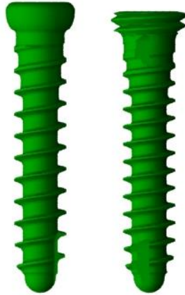
Figure 2.10: Standard non-locking (left) and locking screws (right). The locking screw has a threaded head, which locks in the plate, while the non-locking screw has no feature on its head. (OrthoHelix Surgical Design, Inc) (pending copyright approval)
