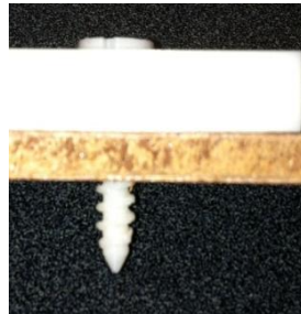
Figure 4.6: Flush fit between rapid prototyped fixation system and wooden bone analog.
