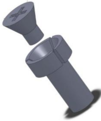
Figure 2.16: Nested screw design: The smaller, inner screw is inserted in the larger screw, causing the outer to expand into the plate. (Song et. al, 2011)
