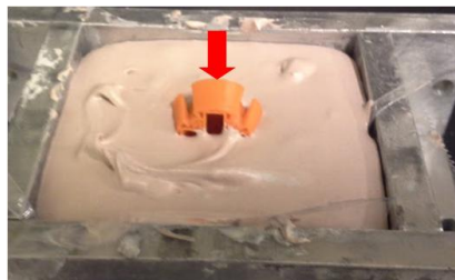
Figure 4.18: Cemented screw head. The red arrow represents the compressive force applied.
