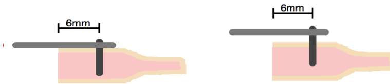
Figure 5.3: Schematic of cyclic loading testing. (a) Set-up of cyclic loading tests with plate flush to the bone model (b) Set-up of cyclic loading tests with plate 2mm above the bone model.
