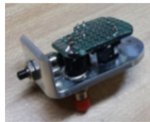
Figure B10: Switches soldered onto a protoboard and mounted
