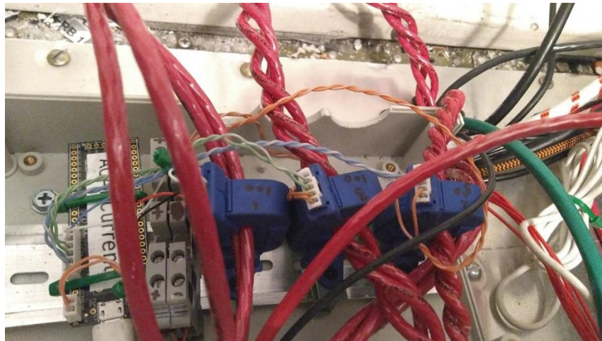
Figure C4: Current sensors and the Cypress PSoC 5LP microcontroller
