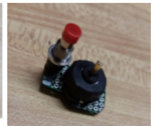
Figure B11: Shrink Wrap around the 5-way switch
