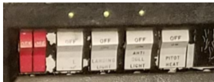
Figure B17: LEDs over Master Switch panel
