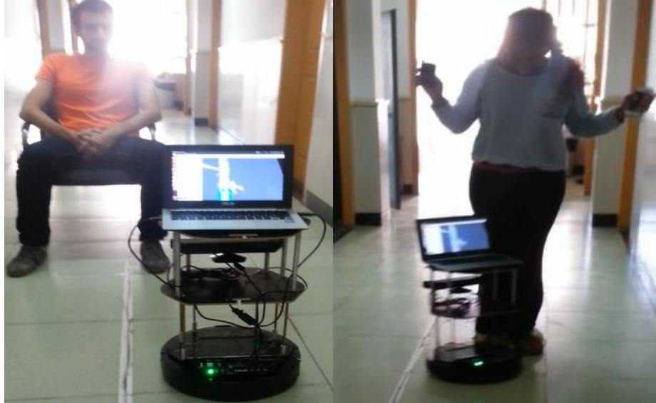
These images above show how the turtlebot can avoid obstacles in its environment.
