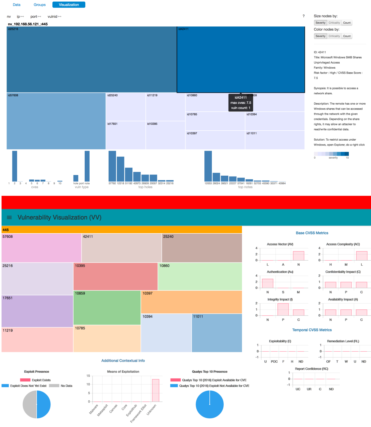
Figure 5.3: Side-by-side comparison of a deep level treemap view of the NV tool (top) and VV tool (bottom), separated by the red line. At this point, the NV treemap cannot descend any further. The NV tool shows all the vulnerabilities for the given port, and details can be viewed via mouseover. The VV tool goes one level deeper, and allows viewing of a single vulnerability, where details are shown in the treemap box. Also, context charts update to represent the data currently in view for the VV tool. The NV tool bar charts do not change in this manner.
