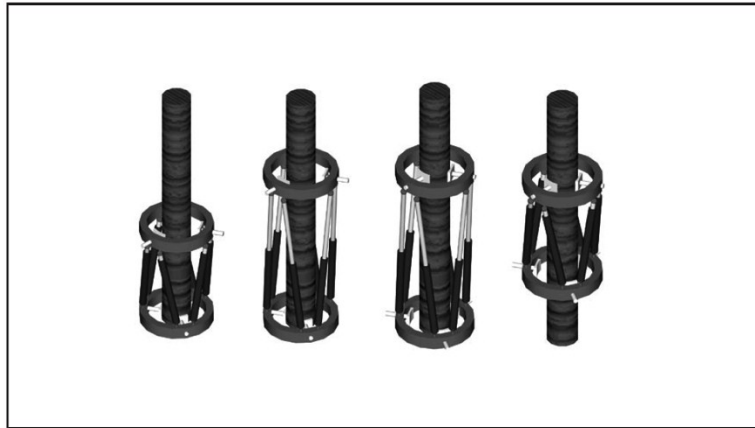
Figure 9: The Four-Cycle Climbing Steps of the TREPA Parallel Climbing Robot
