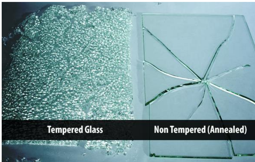
Figure 2: Fragments of Tempered vs. Non-Tempered (Annealed) Glass Plates
