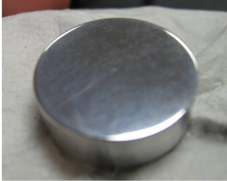
Fig. -. The sample in which we are going to indent which has a surface roughness of 0. 050 microns.
