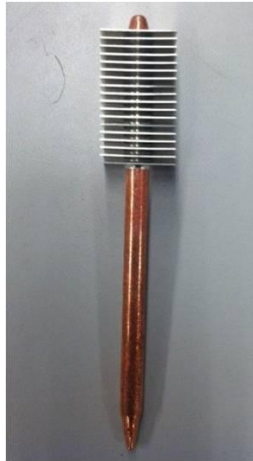
Figure 46: Close up picture of heat pipe
