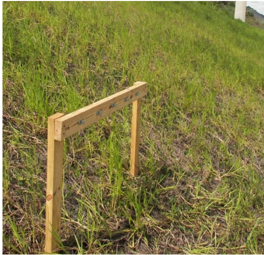
Figure 17 - Soil erosion bridge installed at site 2 which features hydroseeding (Photo Credit: Bryan Lee, 2011)
