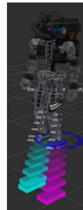
Figure 2.6: The planned steps for the robot walking forward and to the left
