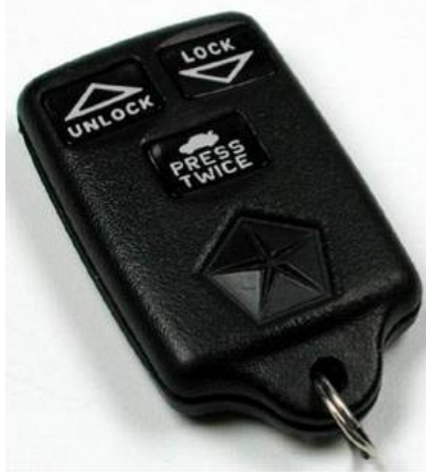
Figure 13 Example image for what a key fob looks like [34]. Usually these have the standard buttons for unlocking and locking doors, opening the trunk, and panic button.
