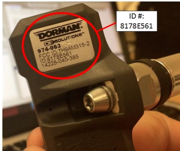
Figure 42 DORMAN TPMS module, ID number 8178E561.
