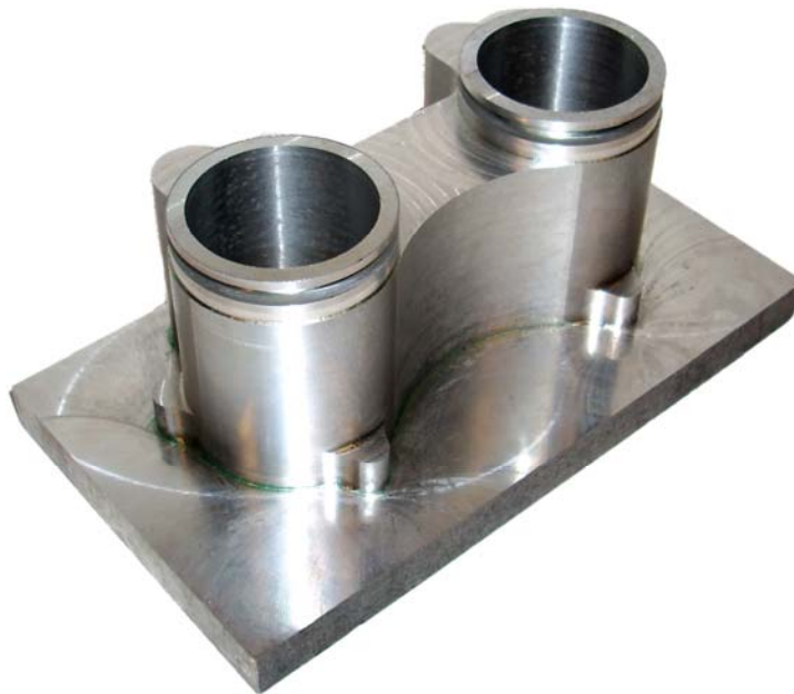
Figure 11: Unfinished New Injector Manifold
