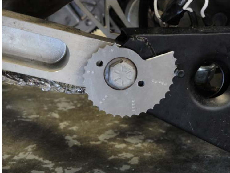
Figure 2: Final Swing Arm Adjust Installed
