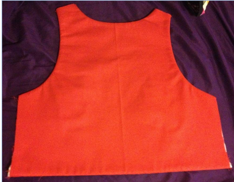
Figure 54—Back of vest sewn, flipped right side out, and ironed
