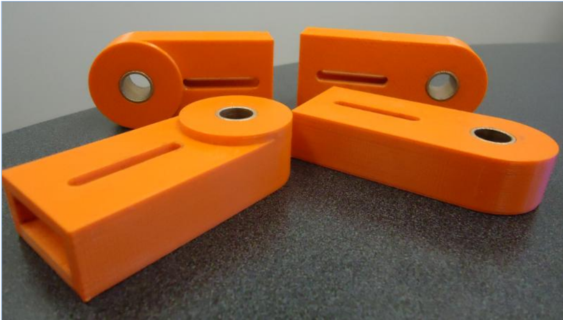
Figure 47—Parts created using rapid prototyping
