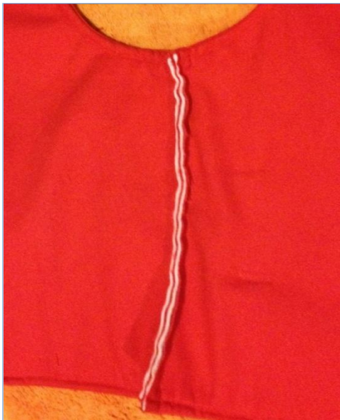
Figure 56—Side sewn to back of vest
