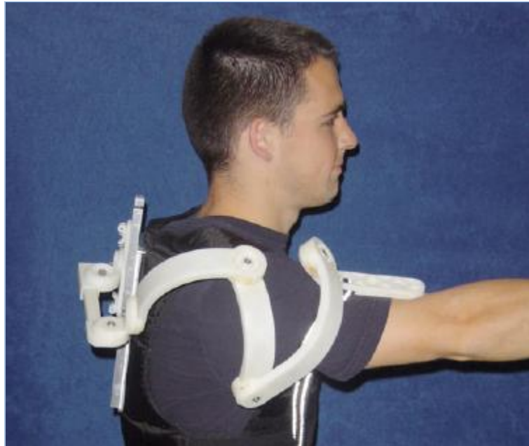
Figure 12—Prototype of powered upper limb orthosis (Carignan et al., 2005)
