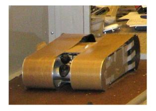
Prototype 2 with the wheels taped so they can not move. This was done for a friction test of the belts.
