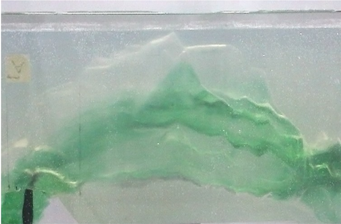
Figure 6.8 Dye visualization in pre-op nasal model during expiration.
