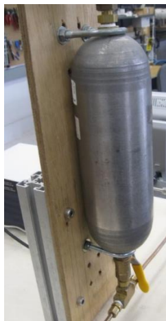
Figure 11: Fluid Reservoir Assembly
