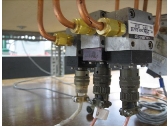
Figure 12: Undermounted EHD Differential Pressure Transducers
