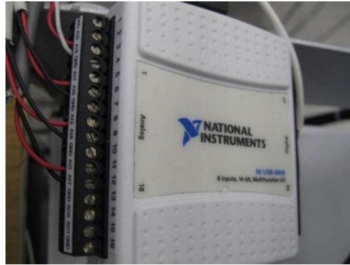
Figure 14: NI USB-6009 Data Acquisition Configuration
