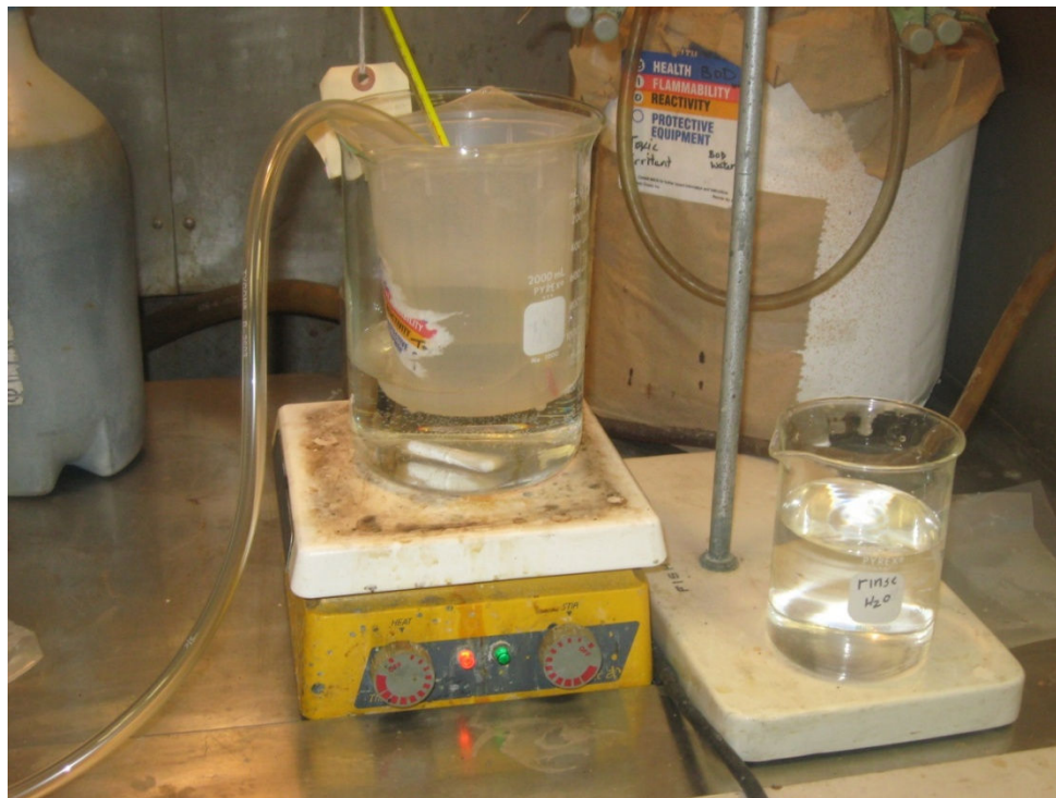
Figure 5: Laboratory setup for scaled down hydrofluoric acid bath
