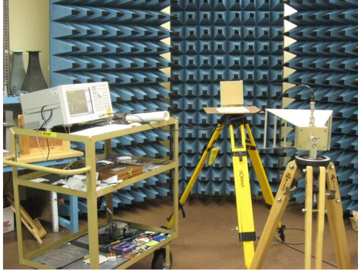
Figure 37. Measuring S21 of our aperture coupled patch antenna
