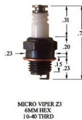
Figure 41: Rimfire spark plug (Rimfire).
