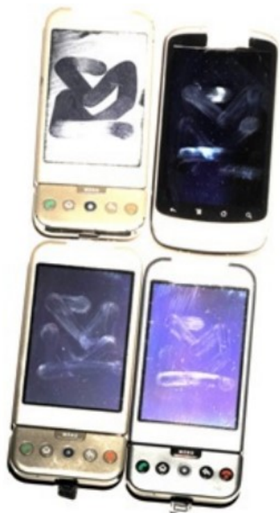
Figure 2: Residual oil patterns on smartphone screens are visible, even without optimal lighting [3]
