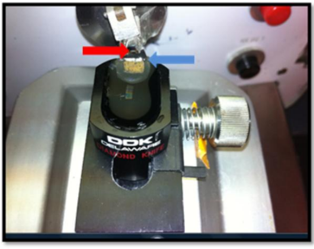
Figure 4: Cutting of Muscle Tissue Sample on Microtome. The block of resin (red arrow) in a metal chuck is carried by the microtome mechanism past the stationary knife (blue arrow).
