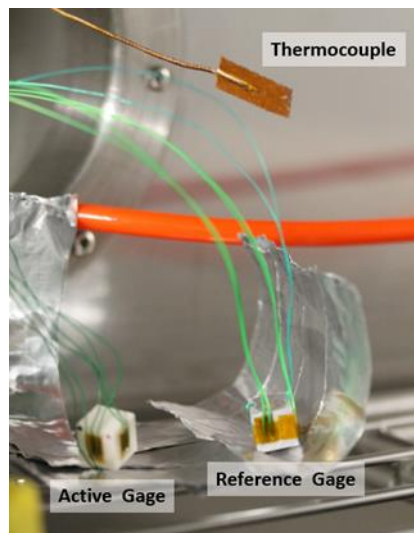
Figure 3-2: Image of thermal test set-up
