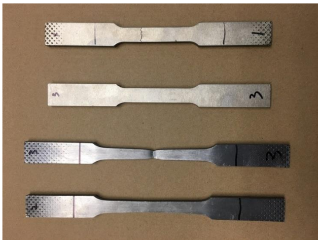
Figure 39. Two sets of specimens: tungsten alloy and lead alloy. For each set, the upper one is the tested and the lower one is the unused.
