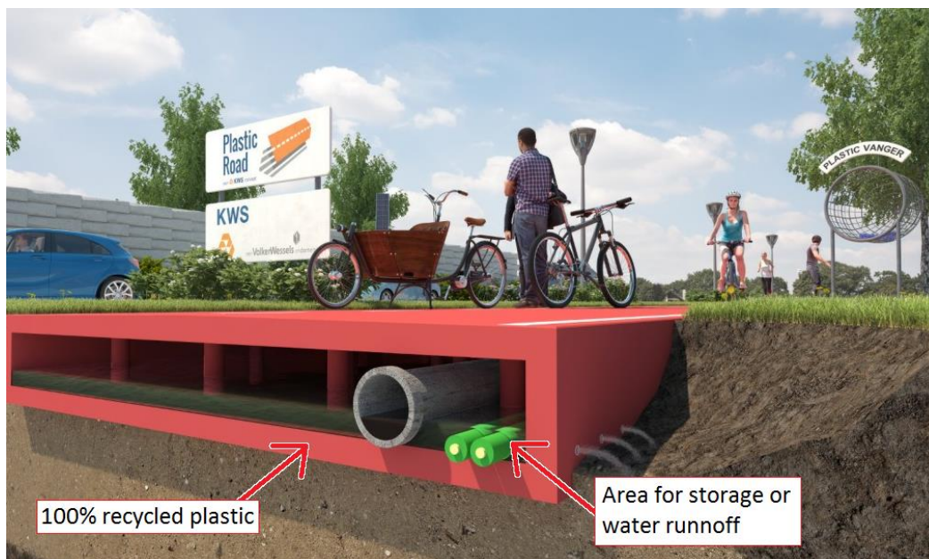
Figure 10: An artist's rendition of VolkerWessels Plastic Roadway. The road is made of 100% recycled plastic and is totally module [29].
