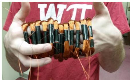
Figure 28: Our twelve coils are shown here. Each of them is three-hundred turns of 28 AWG copper wire.
