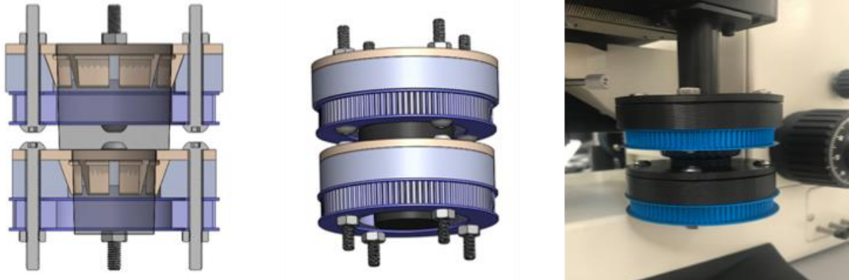
Figure 18: Design III - CAD Models of the X and Y Axis Dial Adapters (left and middle) and Final Dial Adapters (right)
