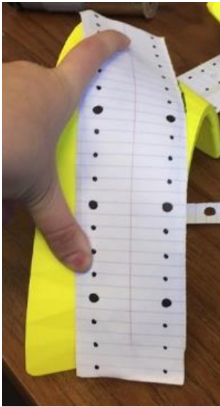
Figure 38: First iteration of shoulder pads with template for hole drilling
