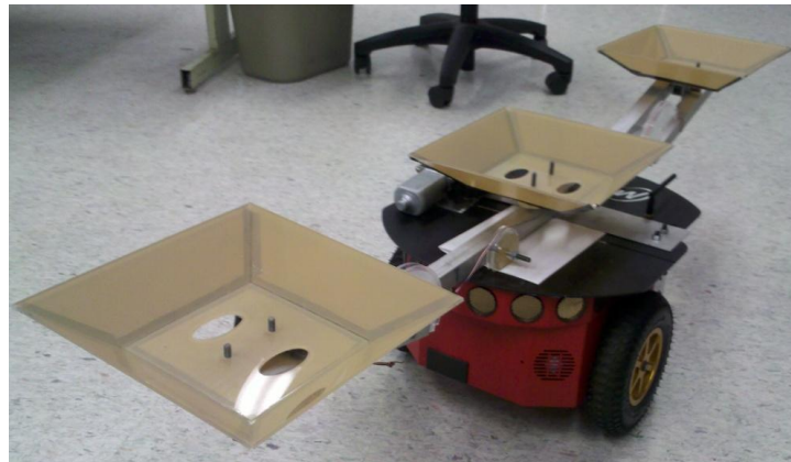
Figure 47: UGV with landing platforms in the deployed position
