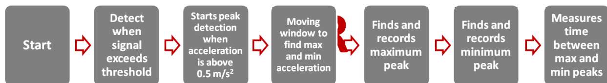
Figure 77: Block Diagram of Final Design.
