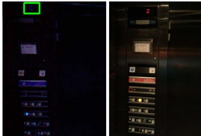
Figure 49: Kinect Positive recognition of the second floor from the LED screen in the elevator (left) and scene from non-Kinect camera (right)
