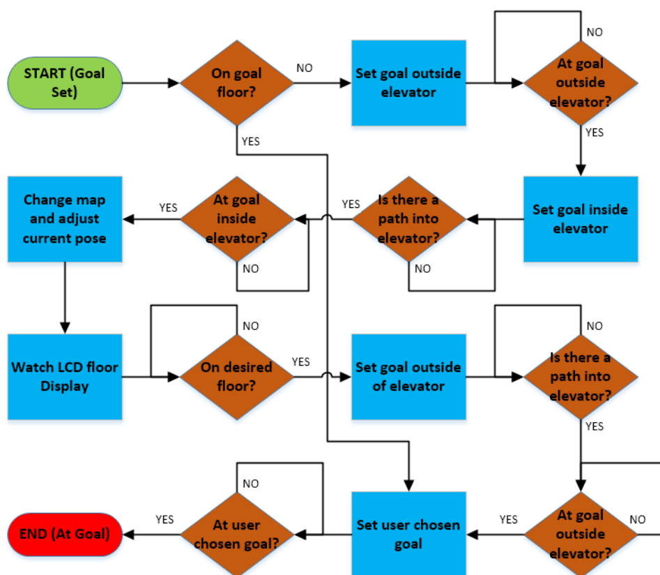
Figure 53: Multi-floor planner elevator protocol flow-chart
