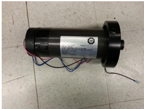
Figure 12: Proform Power 990 Treadmill Motor
