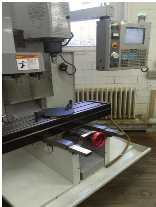
Figure 25: Motor Sprocket on the CNC machine
