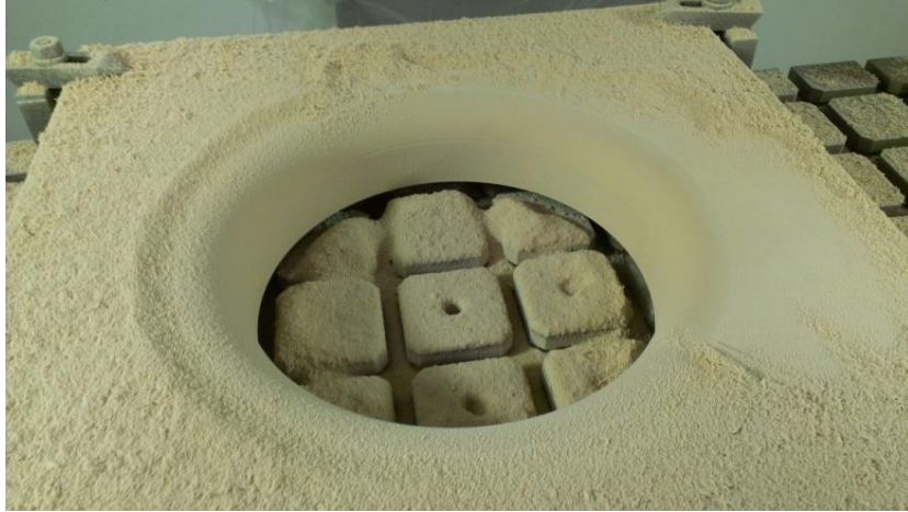
Figure 24: VM3 CNC with Tooling Board Bell Mouth
