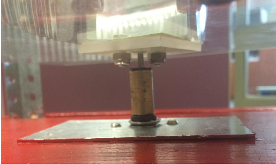
Figure 3-4: Shaft Collar Connecting the Turbine and the Generator
