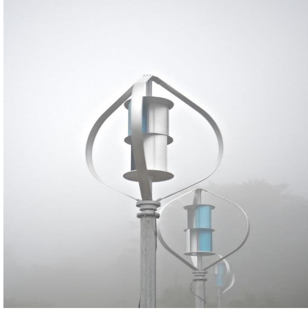
Figure 2-5: Darrieus Wind Turbines With Savonius-Type Start-Up Rotors
