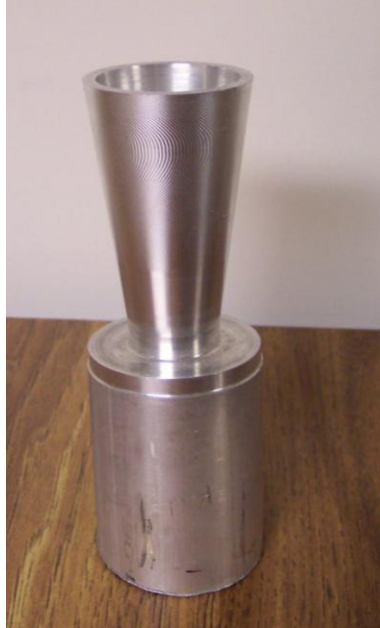
Figure I.1 Restrictor inlet cone with extra stock, complete.
