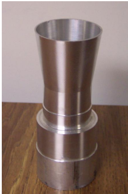
Figure I.4 Plenum cone, completed.
