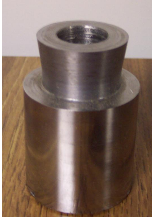
Figure 9.12 Partially machined turbine inlet cone.
