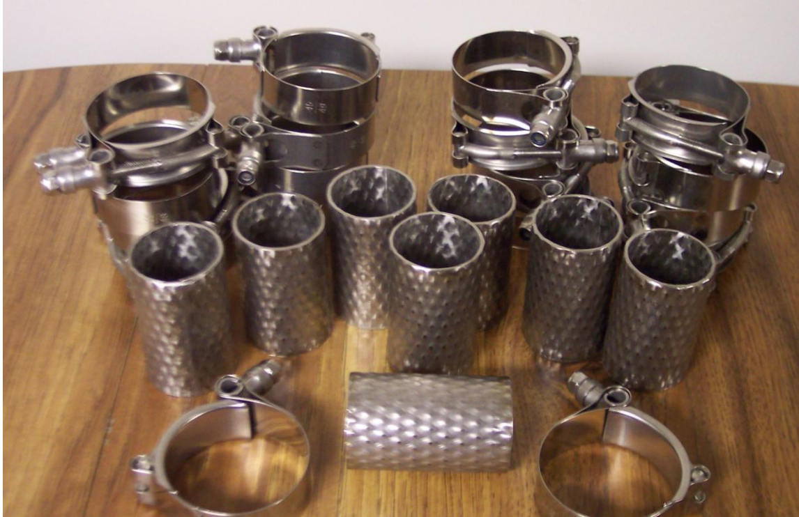
Figure I.13 Clamps and joiner for 1.5 inch ID silicone hoses.
