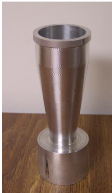
Figure I.2 Restrictor outlet cone with extra stock, incomplete.
