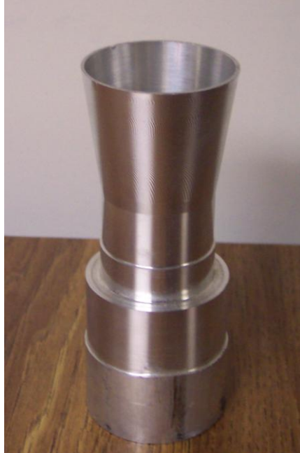
Figure 6.13 Completed plenum cone.
