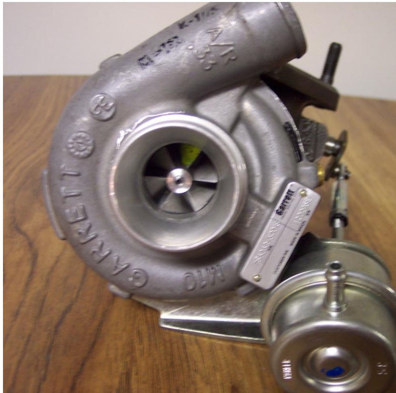
Figure D.3 GT12 Turbo, compressor inlet.
