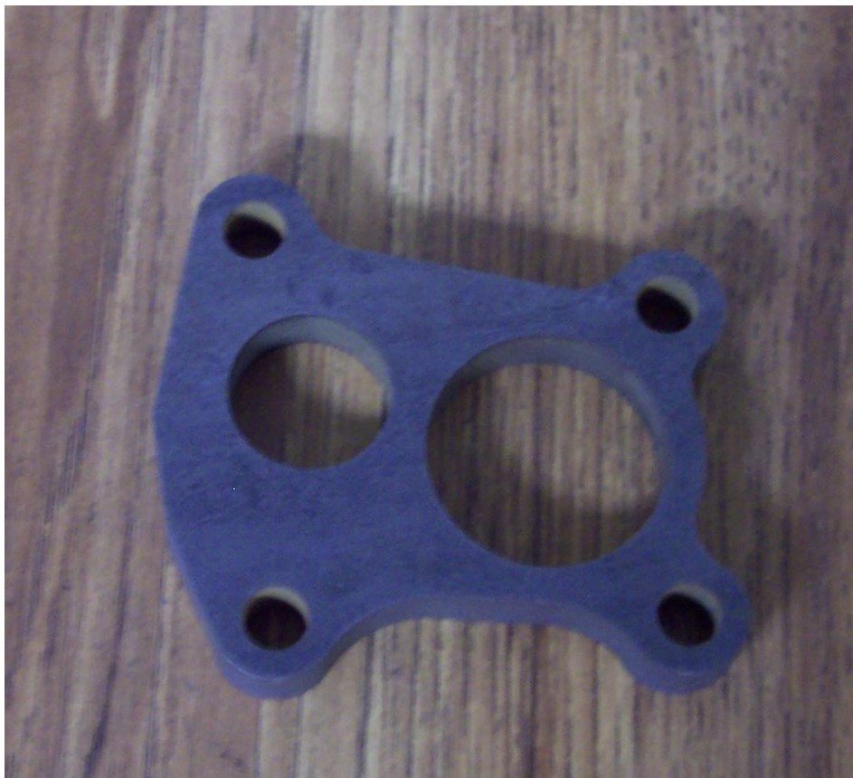
Figure 9.10 Steel turbine outlet flange.
