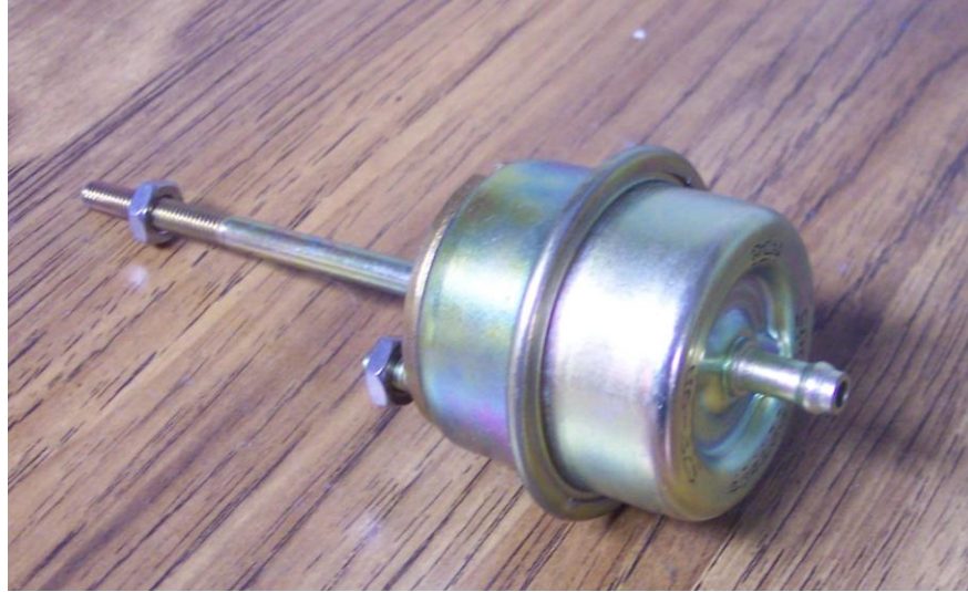
Figure 8.14 18psi integral wastegate actuator.
