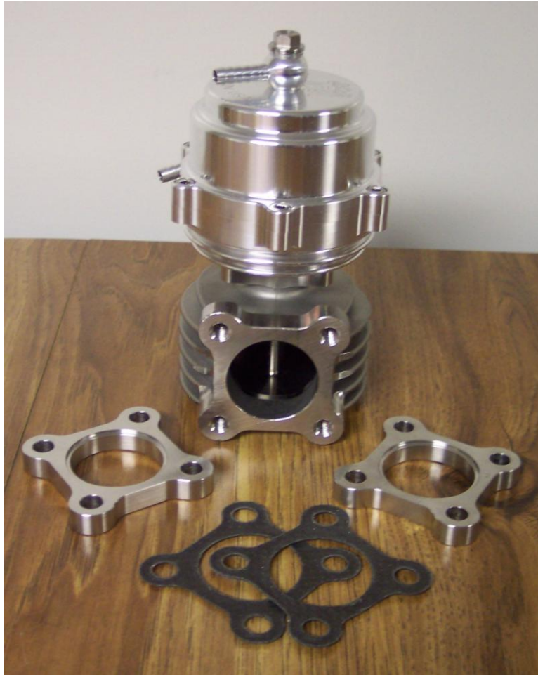
Figure 8.13 TiAL F46 remote wastegate with flanges and gaskets.
