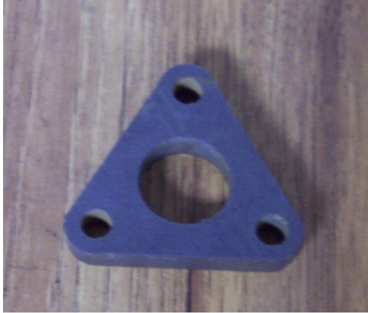
Figure 9.9 Steel turbine inlet flange.
