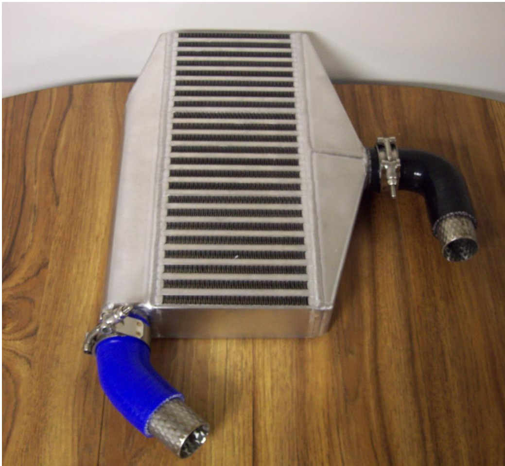
Figure I.16 Intercooler with silicone hoses affixed to it.
