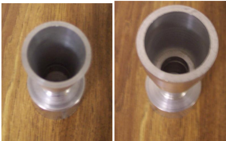
Figure 6.7 Restrictor inlet (left) and outlet (right) cones.
