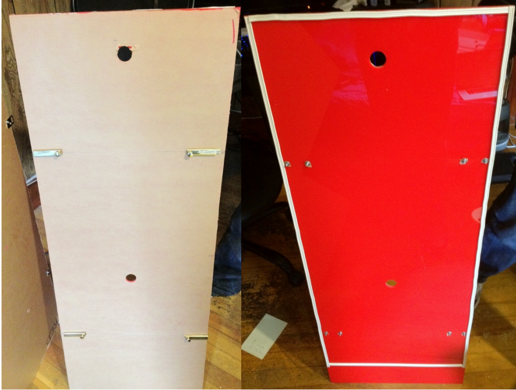
Figure 13: Enclosure Back Door and Sealant Placement
