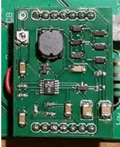
Figure 5-15: The Power PCB Mounted – Component View
