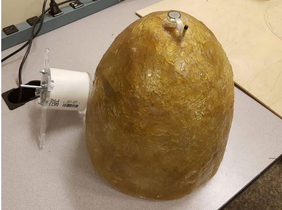
Figure 5-33: The Formed Fiberglass Nacelle Shell
