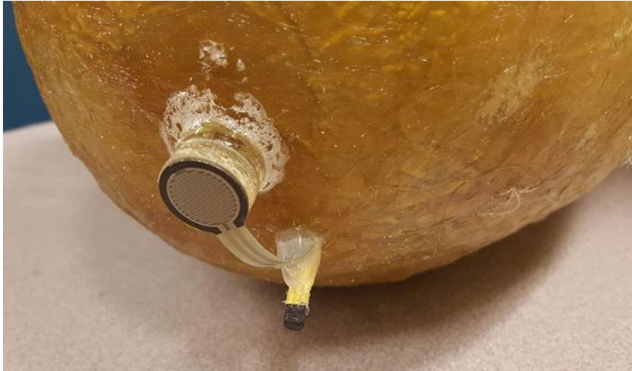
Figure 5-34: The Nose of the Nacelle Shell, with the FSR and TMP36 Visible
