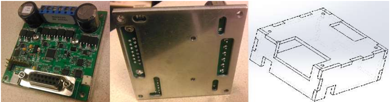
FIGURE 19: MOTOR CONTROLLER BOARD, LEFT COMPONENTS AND PORTS, MIDDLE HEAT SINK PLATE, RIGHT PROPOSED DESIGN FOR CASING
