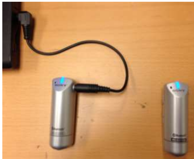
FIGURE 21: THE MICROPHONE AND RECEIVER UNITS
