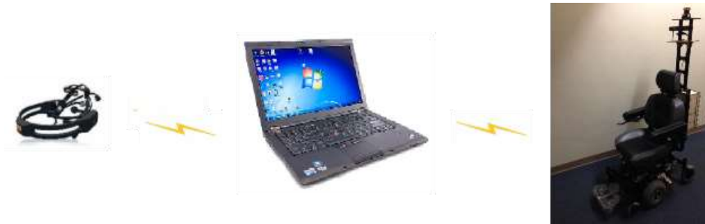
FIGURE 24: HARDWARE SETUP AMONG HEADSET, COMPUTER AND WHEELCHAIR
