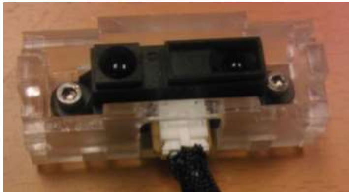
FIGURE 5: IR SENSOR TRAPPED INSIDE OF ASSEMBLE CASING
