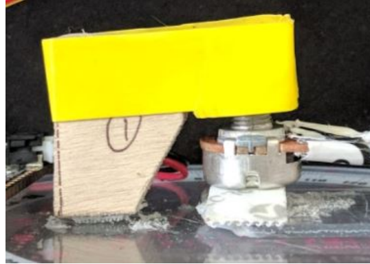
Figure 7.8. Side view of wooden “arm” for potentiometer fixation on electric goniometer.
