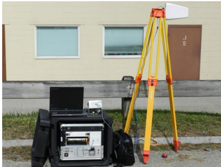
Figure 51: A photo depicting one entire receiver setup for the time difference of arrival (TDOA) system. The analog to digital converter (ADC) and the field programmable gate array (FPGA) card are in the black case, the antenna is mounted on the survey stand, the control center is the laptop, and the GPS disciplined oscillator (GPSDO) is in the metal box next to the laptop.
