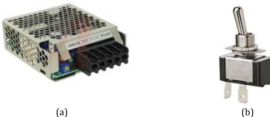
Figure 23: (a) A DC power supply rated at 12 V and 2.5 A. (b) A power switch used on the outside of the enclosure.
