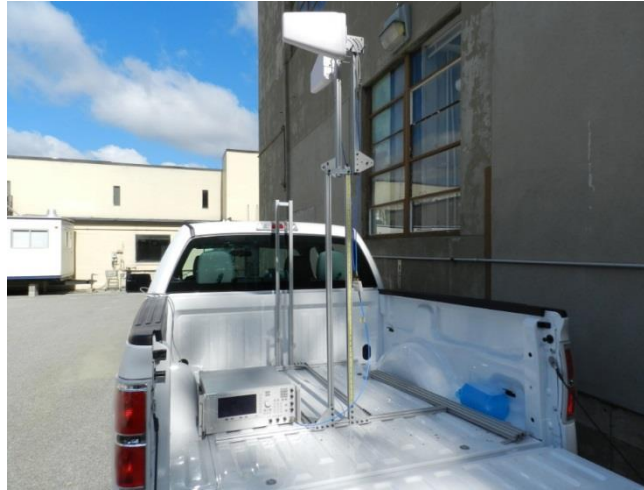
Figure 52: Picture of the transmitter used for field-testing the time difference of arrival (TDOA) system.
