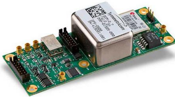
Figure 19: Microsemi GPSDO 2650 used for clock synchronization.
