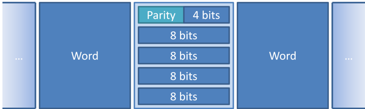
Figure 3-1. Original Data Format as Extracted from SRAM. Each word consists of 5 rows of 8 bits each. The first row of each word contains the parity bits from the SRAM as the first 4 bits of the byte. The remaining 4 bits are the first 4 bits of the 32-bit word.
