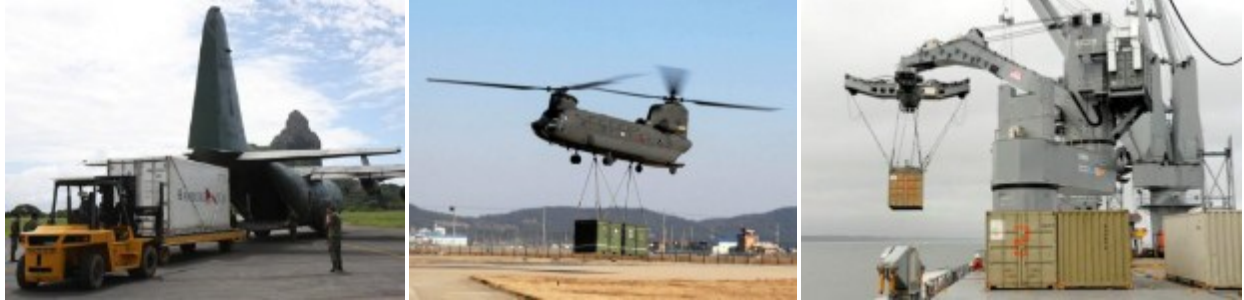
Figure 7. Typical methods of container transportation, such as a C-130 [22] (left), a helicopter sling load [23] (center), and a ship-mounted crane [24] (right)
